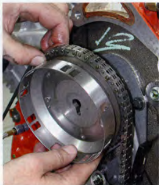
Rotate the engine over to line up the timing marks of the cam and crank gears, and then remove the cam drive gear. The sheetmetal wheel attached to the cam gear signals the cam position for the ECU.
