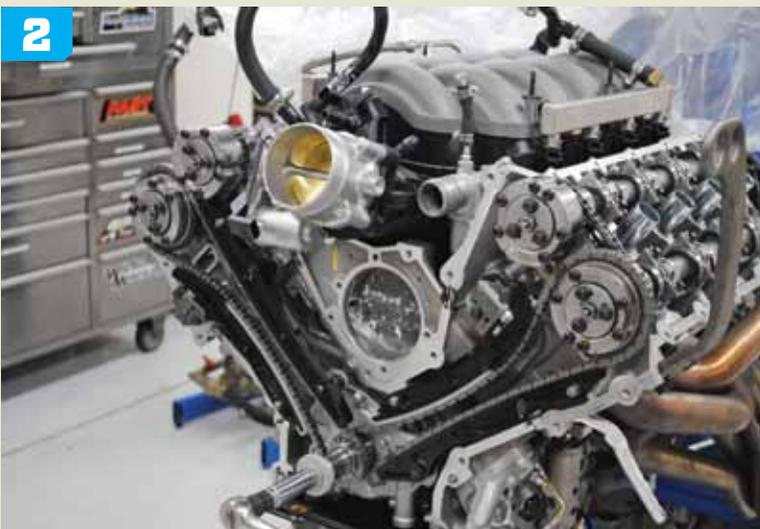
**2** Off came the factory damper, Meziere electric water pump, and front cover to allow access to the timing chains, tensioners, and cam phasers.
