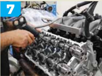
With our cam phasers off, we slowly removed the cam towers, then with all the bolts loose, we used the electric gun to spin them the rest of the way off. They must be removed a half turn at a time to evenly release spring tension from the cam and towers.
