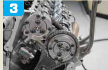
**3** These are the magic cam phasers that allowed the cams to rotate independently of the sprockets. The three center bolts secured the phasers to the cams, while the outer Torx bolts secured the cover plates on the phasers.
