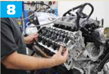
With the towers removed, off came the factory cams. Though equipped with variable cam timing, the stock cams were pretty tame.
