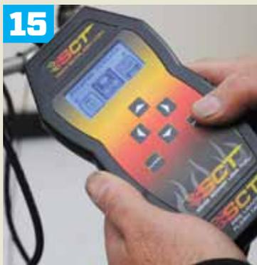
Cam installation required programming to optimize performance. A big thanks goes to Ken Christley at Kenne Bell for his help. Once the tune was finalized, it was supplied to the hand-held unit for loading in the factory computer. The X3 Power Flash from SCT was also used to data log the variables during each run. That data was used to facilitate further tuning.
