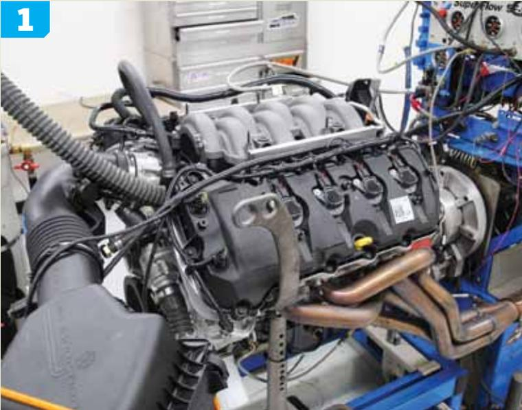
**1** Our test mule was a Coyote crate motor supplied by Ford Racing Performance Parts. FRPP also supplied the Controls Pack that included the necessary components to get the crate motor running. After adding long-tube headers from American Racing Headers, the 5.0L produced 462 hp and 411 lb-ft. This served as our baseline for the cam test.
