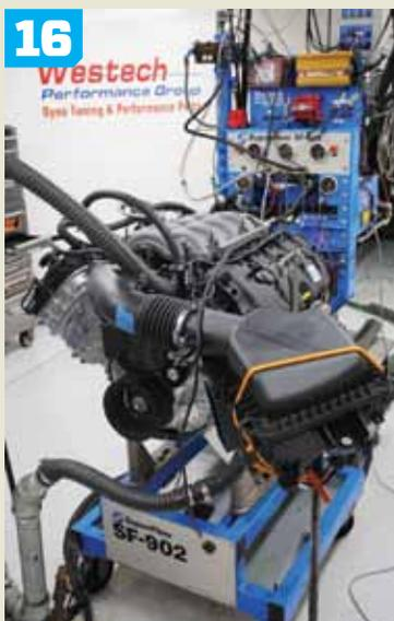
Run with the new Comp Stage 2 cams, the 5.0L Coyote produced 498 hp and 441 lb-ft of torque—up from 461 hp and 410 lb-ft. Those are serious gains from a simple cam swap.
