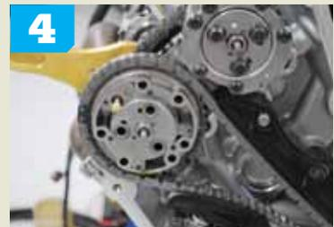
**4** It was necessary to remove the cover plates to install the phaser limiters. Note the small spring and star-shaped plunger. Make sure not to lose these when removing the cover plates and that they are in place after installation of the limiters.
