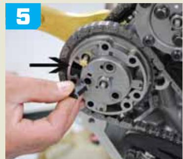
**5** The kit included four phaser limiters, one for each head. The limiter was installed in the opening between the inner and outer sections of the phaser directly below the star-shaped plunger (arrow).
