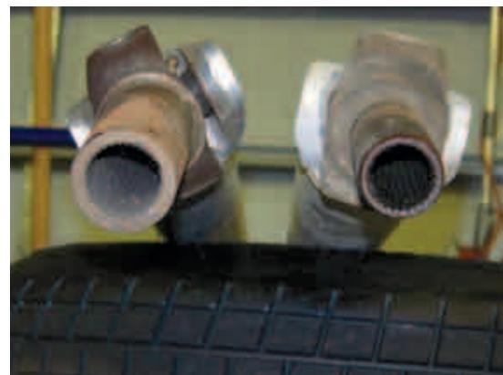
Different transmissions use different size output shafts. Make sure you give your driveshaft manufacturer an accurate spline count for the yoke because they can vary, as you can see here.
