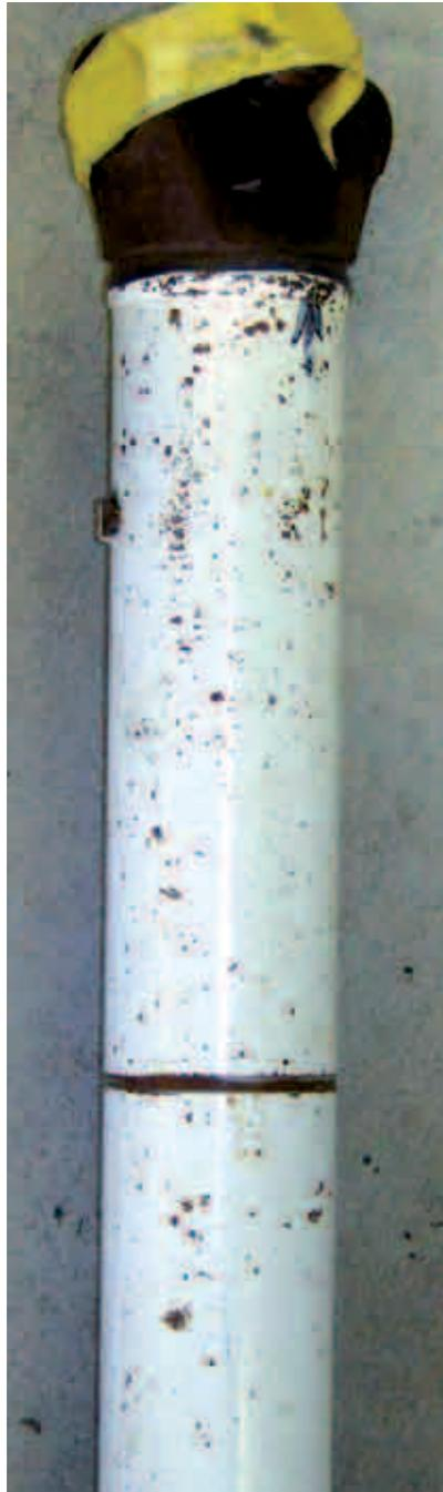
Here's a good example of a driveshaft that's ready for the trash bin. Something happened during a race to cause some other component of the race car to come into contact with the tubing. When whatever it was came into contact with the rapidly spinning shaft it didn't take long to create a groove that will significantly weaken the shaft.
