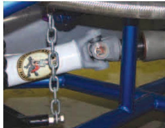
When the driveshaft is installed, make sure you have between  $\frac{3}{4}$  to 1 inch of free play before the slider yoke bottoms out on the transmission's output shaft with the car at ride height.
