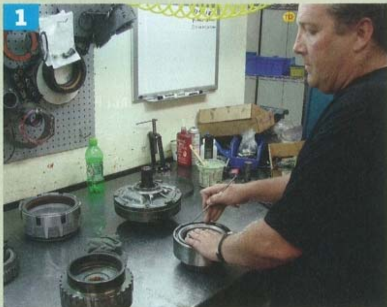
TCI transmission technician Paul Wilbanks, a 20-year TCI employee, starts assembly by assembling the forward drum.
