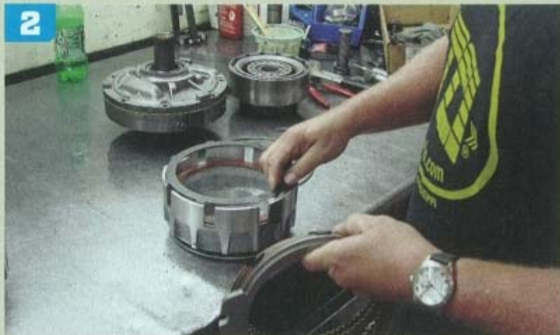
He then installs the clutches into the Fourth clutch assembly.
