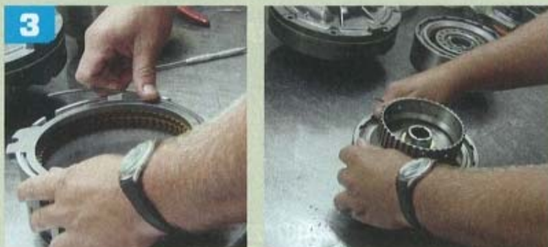
Using a lock ring, Wilbanks locks the clutches into place.
