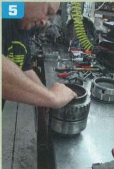
He then installs the direct clutch hub onto the direct clutch assembly.
