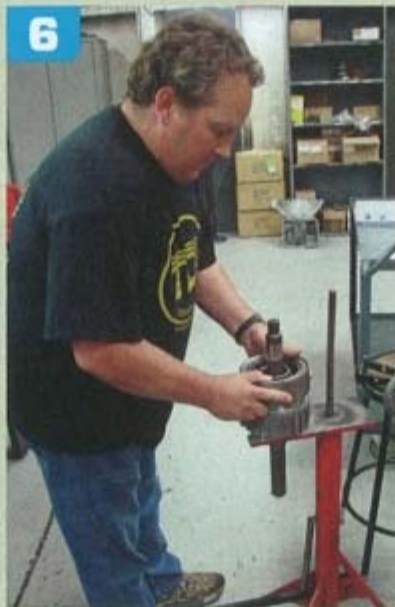
Using a jig, Wilbanks slides the components together one piece at a time.
