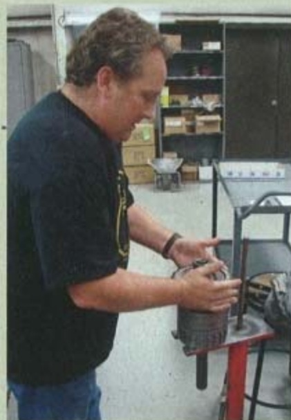
Using a jig, Wilbanks slides the components together one piece at a time.
