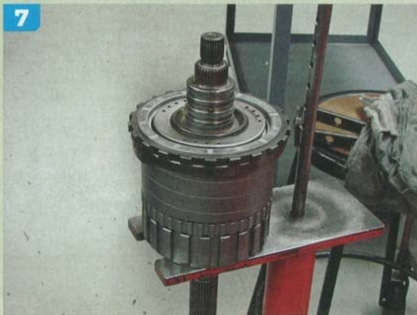
Once assembled, the internals will be lowered into the transmission housing.
